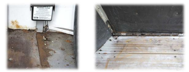
Remove mats and check condition of floor. Pay special attention to corners where moisture may accumulate. These two photos show a trailer with steel frame and wood plank floor. Corrosion is visible on steel components with rust holes in some areas of frame along bottom of side wall. Rust damage of this nature affects the trailer's structural integrity.
