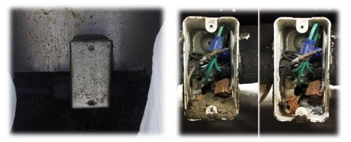
Some trailers have junction boxes, for brake wiring, installed between the axles. Check that these boxes are covered and tightly sealed. If they are not tightly sealed, dirt and water will get into the boxes and cause wiring corrosion which can affect proper brake operation. Photo at right shows same junction box before and after it was cleaned out.
