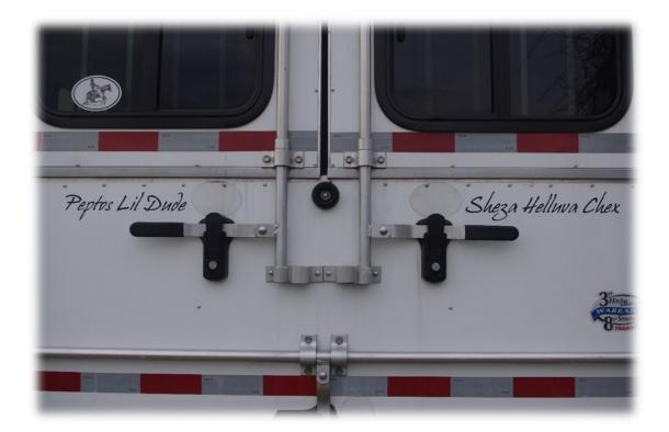
Check all latches for condition and smooth operation. If keyed locks are fitted, lubricate them to prevent seizing. Use a graphite lubricant for keyed locks to keep dirt out of the mechanism.
