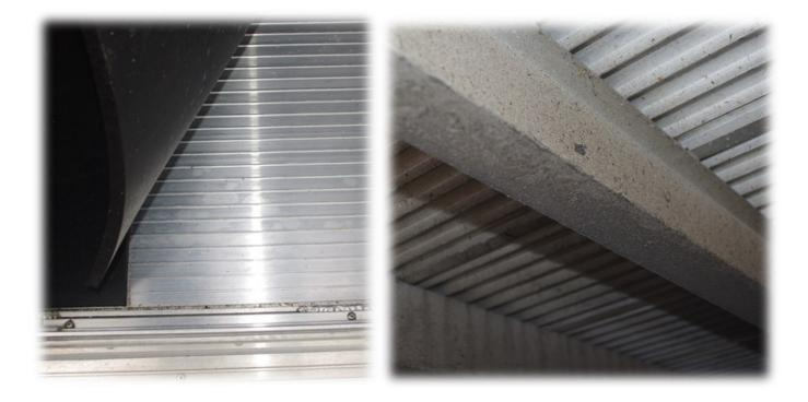
Interior and exterior views of floor and frame on an aluminum trailer. Preventive maintenance, in the form of regular "deep cleaning" of your trailer combined with keeping it dry inside, will help keep your trailer's floor in good condition. Another form of preventive maintenance which will protect the exterior of your trailer's frame and floor is an annual oil spray (often referred to as "rustproofing") which is a worthwhile investment to make in any trailer, used or new.
