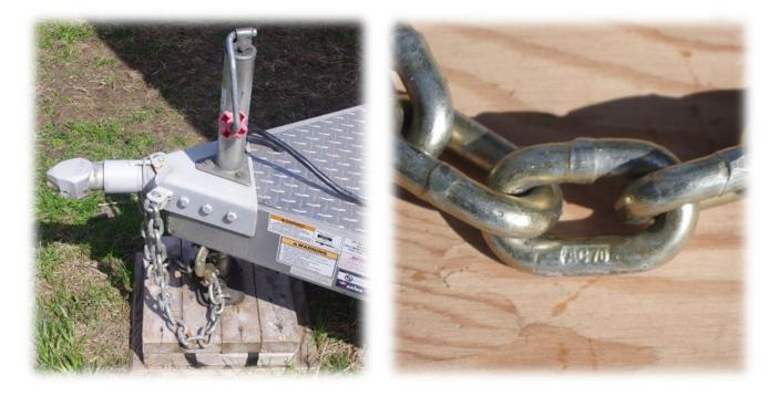
At front of trailer, check condition of the trailer coupler and attachment to trailer frame. Left photo shows coupler bolted to an aluminum trailer. On steel trailers, coupler may be welded in place. Inspect the jack and safety chains. Safety chains should be in good condition and of the proper grade – look for a marking similar to the "AC70" shown (above, right).
