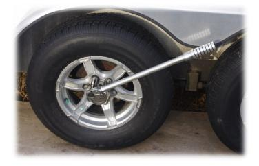
A specialty tool worth purchasing is a torque wrench. Trailer axles do not steer, so every time you turn a corner the tires and wheels are dragged sideways. Over time this can lead to lug nuts becoming loose. Trailer manufacturers advise checking lug nut torque before every trip. The correct torque specification is provided in trailer owner's manual, and may also appear on an information decal. If no torque specification can be located, 90 ft/lbs is a suggested minimum.
