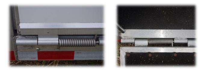
If your trailer has a ramp, look at the condition and attachment of hinges on both inside and outside. Check for smooth operation of the ramp. Corroded hinges will cause the movement of ramp to be stiff and creaky. If the hinges operate smoothly but ramp seems very heavy when you open and close it, look for broken springs.
