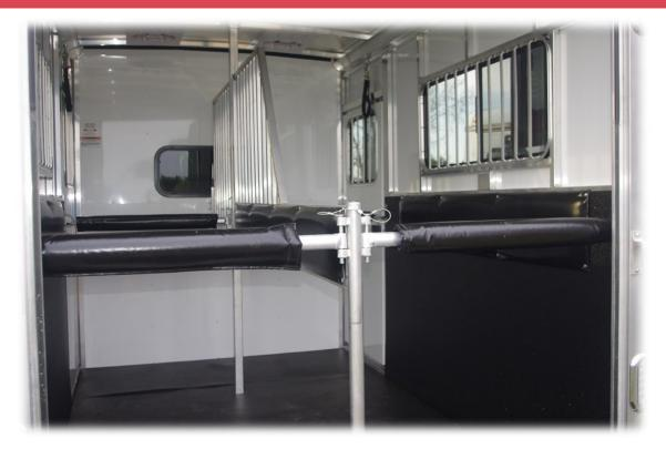
The interior is just as important as the exterior. Inspect the condition of all padding, dividers, tie rings, windows (glass, screens, and latches), window guards, vents, and floor mats.
