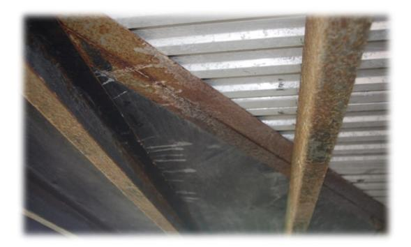
Although the low floor height of most horse trailers can make access a bit challenging, it is important to inspect the underside of your trailer. This one is constructed from a combination of steel frame, plywood floor in tack room and aluminum floor in horse area. Floor panels and frame members all appear to be in good condition with only light surface rust on steel components and no corrosion of the aluminum floor.
