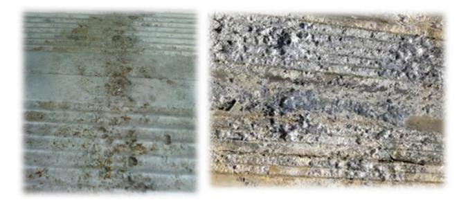
Aluminum does not rust the way steel does, but aluminum does corrode. In a damp environment, pitting corrosion of aluminum often takes place, especially where water cannot travel away from the metal – such as when water (and "other" liquids!) sits between a horse trailer's rubber mats and the floor panels. In photo on left, seam between mats is clearly visible as an area of heavier corrosion and deep pitting.
