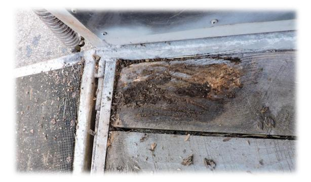
Look for deteriorated floor boards. This floor is in good condition overall with the exception of back corner near the ramp which is an area subject to moisture accumulation. Wood that is beginning to rot should be replaced before one of your horse's hooves breaks through.
