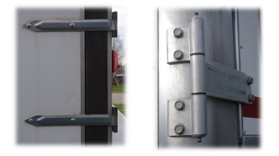
A few drops of light oil on hinges and latches helps to keep them from corroding and becoming stiff. If your trailer's hinges have grease fittings, add a small amount of grease as required and wipe off any excess grease when finished to keep things tidy.
