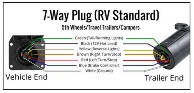
Most tow vehicles and trailers will be fitted with the standard 7-way plug as shown. The functions of each terminal are standardized however wiring colours on your tow vehicle and trailer may be different from the colours shown on plug diagram.
