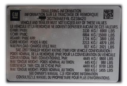
First, the tow vehicle. Shown above is the trailering information decal located on the driver-side door jamb, which includes:
