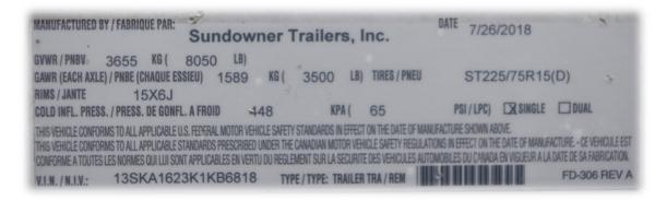
The trailer information decal includes helpful information such as the VIN, wheel rim dimensions, tire size, and tire inflation pressure. The number we are most concerned with here is the trailer GVWR of 3655 KG (8050 LBS), well within the 4445 KG (9800 LBS) TWR for a conventional trailer shown on the tow vehicle trailering information decal.
